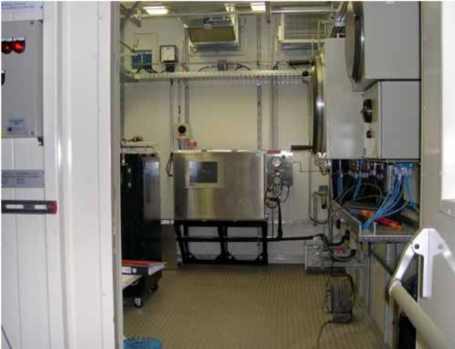
↓ Example of manifold usage for monitoring low level concentration gasses
